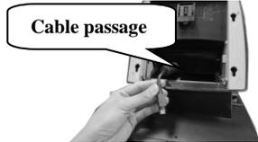
5. After mounting the terminal onto the base stand, connect the cable to the bottom I/O plate of your terminal.
