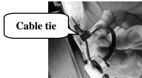
4. Tighten the cable tie again to hold the cables into place.
