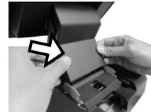
4. Thread the cables along the cable passage and then tilt the screen upwards to pass it through the cable exit.
