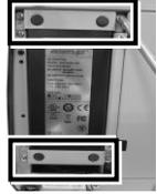
5. Loosen two fixing screws to remove the bracket for the middle compartment.
