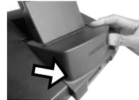
3. Remove the base stand cover by pulling outwards the locking levers with your forefingers and then pulling the cover in the direction shown by the arrow.
