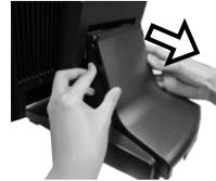
3. Press down the cable tie tab to completely loosen the cable tie.
