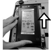
4. Place two brackets separately on the top and bottom sides of the power adapter compartment as shown in the figure. Then, fasten two brackets with four fixing screws.
