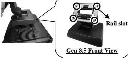
4. Slide the base stand upwards along the rail slot until the terminal is clicked into place.
