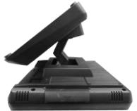
2. Take the AC power adapter with its rubber feet facing you. Place the bottom side of the power adapter into the bottom of the power adapter compartment first, and then push it down into place.
