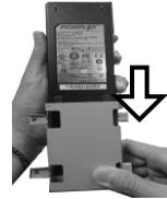
3. Attach the bracket to the wedged portions on the right-hand side of the power adapter compartment.
